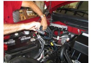
Install the negative ground connector cable (included) to insure that the POWERBOX is making electrical ground contact with the truck chassis. Mount the cable to the exposed grounding bolt on the side of the box near the exposed wires exiting the POWERBOX or to the mounting L brackets on the Chest style unit and then attach it to the chassis of the vehicle. Your POWERBOX must be grounded in order for it to work properly.
