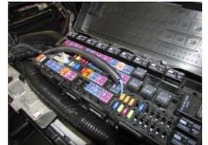
The Blue Control Wire is normally run to the vehicle fuse box and must be attached to a vehicle powered accessory that is only "ON" when the key is in the "ON" position... such as the stereo, cigarette lighter, or any other accessory that is "ON" when the vehicle key is "ON". Some newer vehicles have an accessory slot in the fuse box that provides 12 volt battery power when the key is turned "ON". Please use a volt meter to test the circuitry and verify, prior to hook up.
